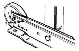
• The dishwasher is shipped to be installed in cabinet opening with a 34" height. Measure height of cabinet opening from the front edge of the underside of cabinet opening to floor. Check chart for that height opening. Put the wheels in the required position. The dishwasher should be installed as level as possible from front to back. Loosen and then turn front levelers the number of times indicated in the chart.
